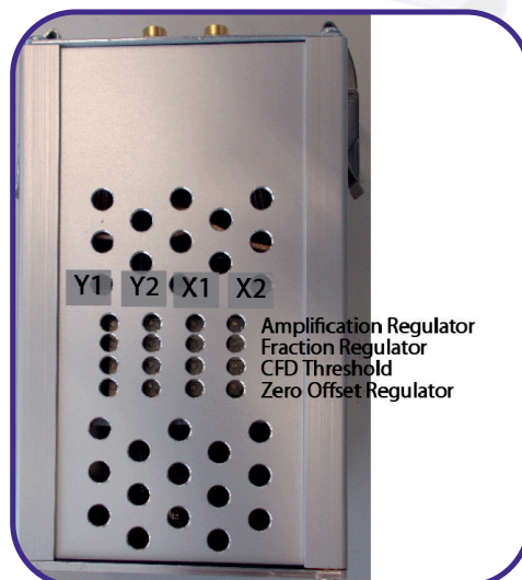
Figure 14: Labelling of discriminator threshold and amplification regulators.
